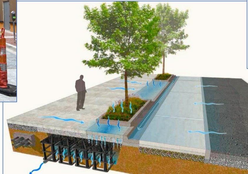
Example of tree cell used to capture sidewalk runoff
