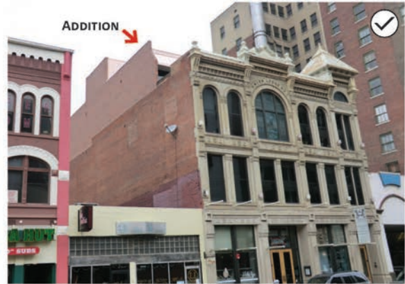
74. Minimize the visibility of a rooftop addition from the street. The building illustrated above has a rooftop addition (right) that is set back and not visible when the building is viewed from the front (left).
