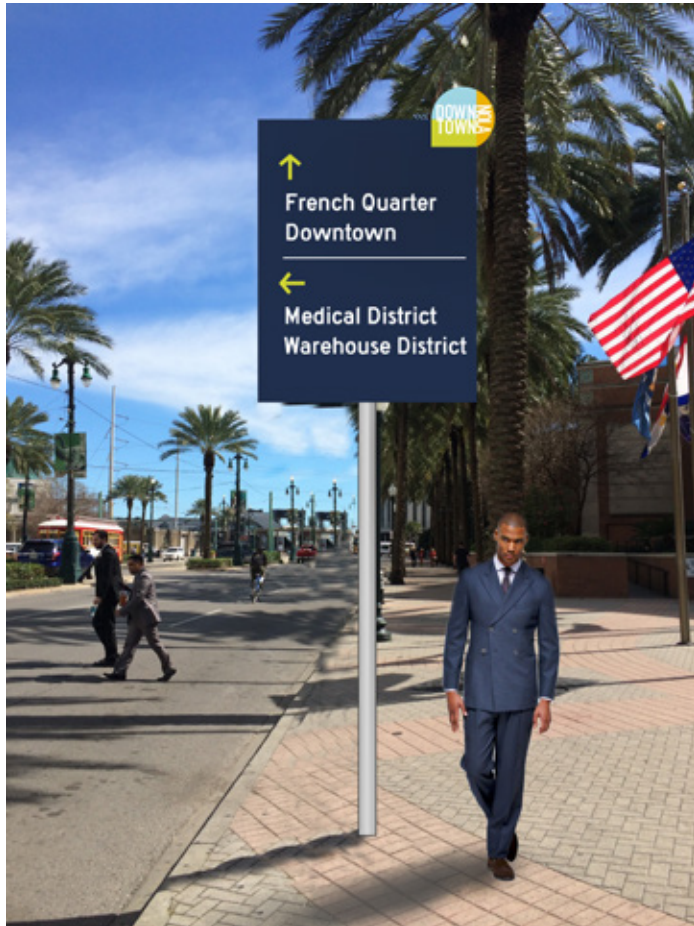
Branded symmetrical design painted aluminium or boxed cabinet. Sign face painted or vinyl colored with retro-reflective sign face.
