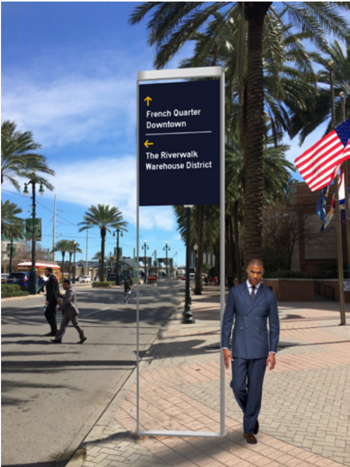
Minimalistic and clean framed symmetrical design with brushed aluminium surround, painted background with retro-reflective sign face per MUTCD requirements.
