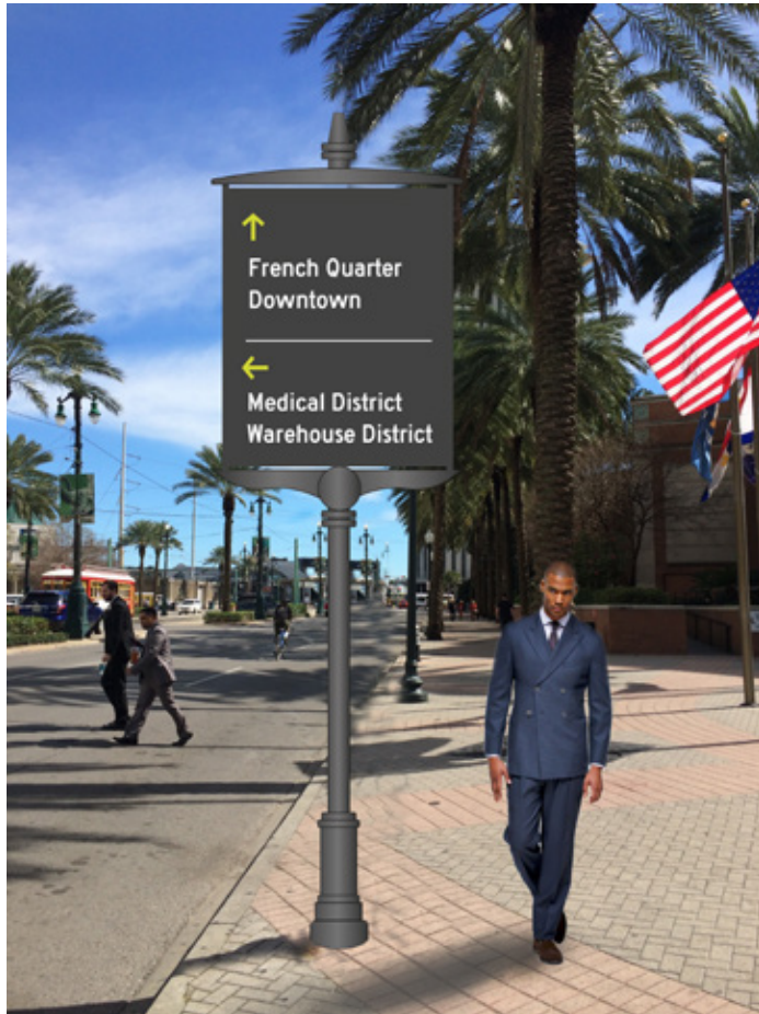
Historic decorative design with district icon painted aluminium on frame-mounted panel. Sign face painted or vinyl colored with retro-reflective sign face.
