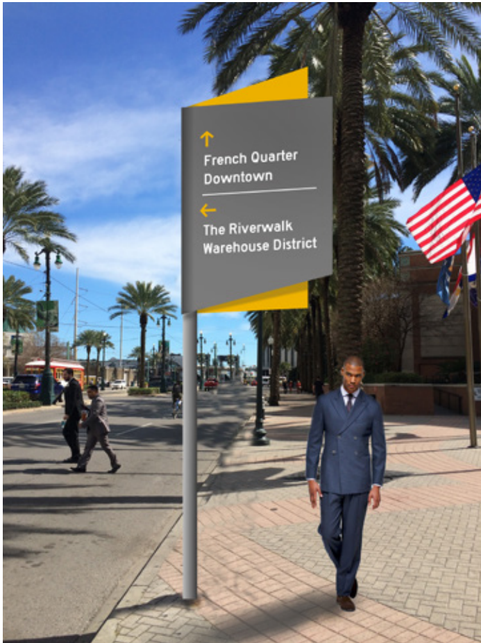
Modern geometric cantilevered design with district specific coloring. Sign face painted or vinyl colored with retro-reflective sign face.
